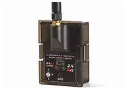
So far, I've connected it to an Orange DSMX, Spektrum DSMX, and a Frsky ACCST receivers. After successful range tests I have flown a quadcopter with each of those receivers to a range of about +1000 feet at an altitude of 200 feet. For shucks and grins, I also connected it to my grandson's toy grade quadcopter, a Sky Viper using the CX10 protocol. In all cases it works just fine.
